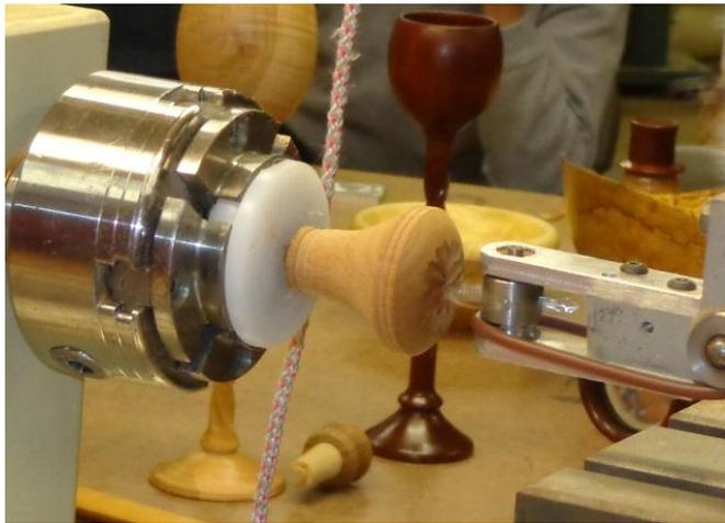
A spinning cutter is brought into contact with a work piece mounted in the head stock. Note the cutter
